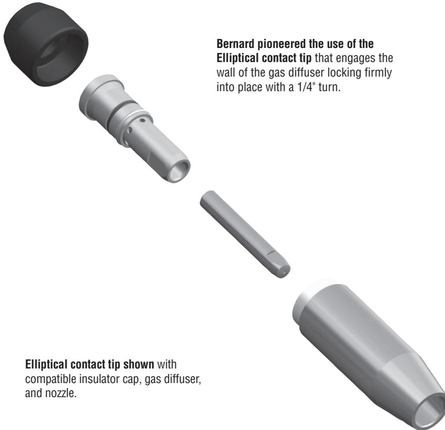
**Bernard pioneered the use of the Elliptical contact tip** that engages the wall of the gas diffuser locking firmly into place with a 1/4" turn.
